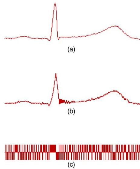
**Fig. 5** Results of ADM techniques: (a) original ECG signal; (b) reconstructed ECG signal; (c) error signal.
