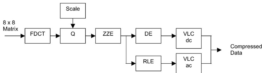
Fig. 1 Block diagram of an encoder. FDCT, forward discrete cosine transform; Q, quantization; ZZE, zigzag encoder; RLE, runlength encoder; DE, differential encoder; VLC, variable length coding; ac, ac coefficients; dc, dc coefficients.
