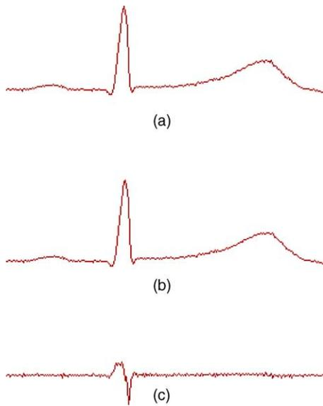
**Fig. 4** Results of DPCM techniques: (a) original ECG signal; (b) reconstructed ECG signal; (c) error signal.
